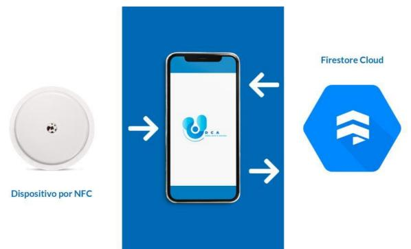
The App is used to connect to the NFC device with Firestore Cloud. This, scans the device and sends the data to the Firestore Cloud at the same time that it shows them in it.
